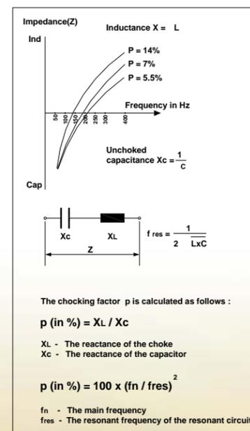
Impedance curve of series resonant circuit Fig.3
